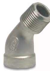
Profec Nr. 121 - Elbow 45° Connection: female thread x male thread Material : stainless steel 316
