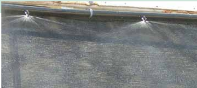
Modular half-circle sprayer 100 l/h mounted every 1.0 m
